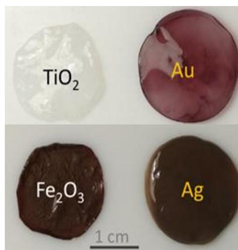
**Figure 2:** Bacterial nanocellulose composited with metal oxide and metal nanoparticles.
