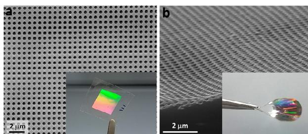
**Figure 1:** SEM of Cellulose based Photonic (a) and Plasmonic (b) crystals. A photograph of each sample is included as an inset for each case; patterned areas are 1x1 cm<sup>2</sup>
