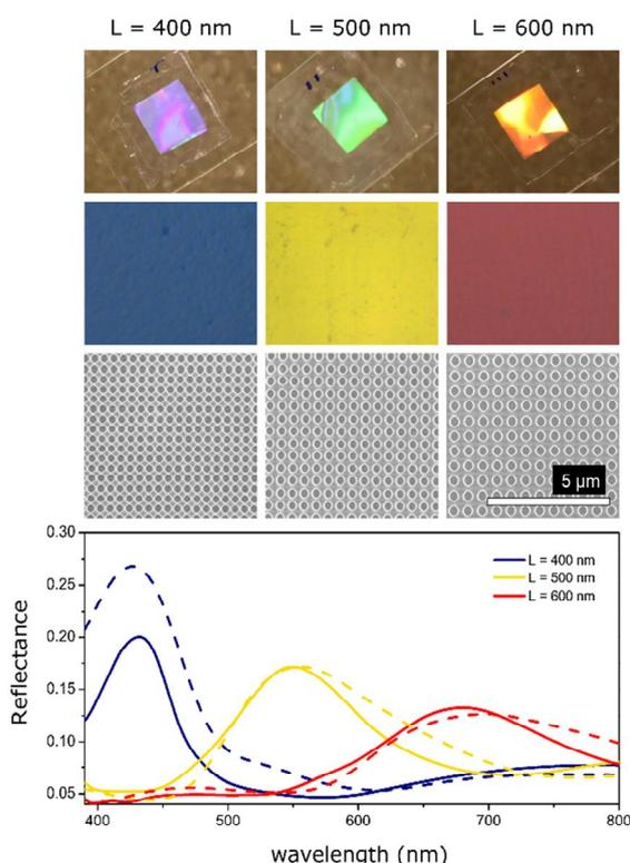
**Figure 2:** HPC photonic crystals present iridescent colours that depend on the lattice parameter of the nanoimprinted structure.
