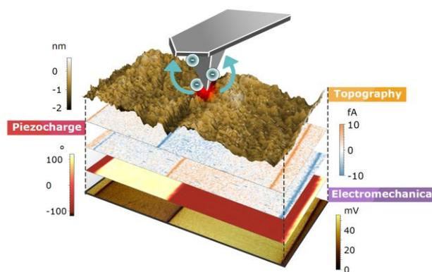
**Figure 1:** 3D rendered image obtained with the full information acquisition: both electromechanical and piezogenerated at the nanoscale are acquired with this new AFM mode.
