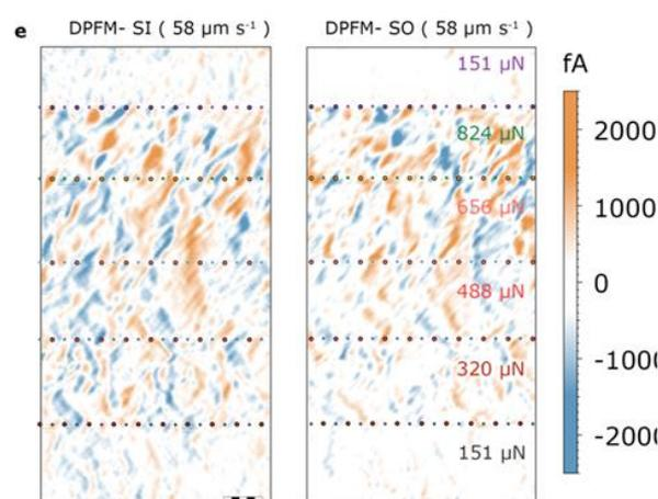
**Figure 2:** DPFM-Si and DPFM-So of a PZT sample acquired by performing DPFM. The images are obtained after a thermal treatment to grown the natural domains structure into the material to study
